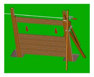
If the screen is placed on grass or other soft surface, make sure that the screen cannot sink into the ground. Support the screen at ground level at 3 places by means of tiles, concrete slab or other hard material.
