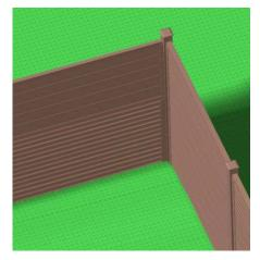
When you want to finish the upper board with a horizontal U-profile (Step 7), make sure that the boards are 5 cm higher than the vertical U-profiles, so that the horizontal profile can be placed onto the upper board. Therefore you will have to cut the vertical U-profiles by 7cm before attaching to the posts (the boards are 200cm high, the U-profile is 202cm long and the vertical U-profile should be 5cm beneath the top board).
