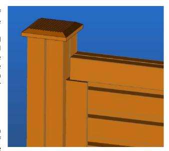
Attach the cover caps after all horizontal U-profiles have been put in place. For posts placed against a wall, the cover cap needs to be cut at one side.
