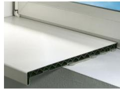
A bed of mortar is provided on the location where the window sill should be installed. The window sill is applied and pressed. The dovetails ensure good adhesion in the mortar. Take into account the drying and curing time before the first use.
