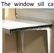
The window sill can be fixed on these saddles at the bottom. First, the saddles are placed on the wall at the desired height, taking into account the minimum distance of 10 cm. (see below) Once the saddles are placed on the wall, the window sill can be secured to the saddles with screws. Make sure that the screws are NOT longer than 16 mm.
